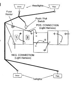
Yamaha Basic 36-Volt Wiring Diagram
